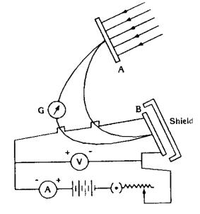
which A absorbs the heat energy is equal to the rate at which heat is supplied to B.
