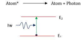
An atom in the excited state may be caused to de-excite by an incoming photon of exactly the same energy. This process of causing an excited atom to return to the lower energy state with the help of a photon of exactly the same energy is called *stimulated emission*. The emission then goes into the same direction as the incoming photon. In effect, the incoming radiation is amplified. This is the physical basis of light amplification in amplifiers and lasers.
